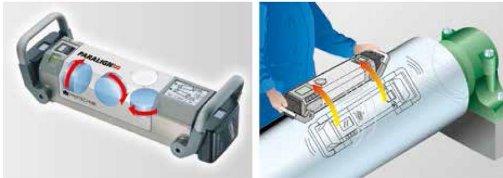
Figure 3: The illustration on the left shows the PARALIGN® measuring device, with the ring laser gyroscopes in blue. Each gyroscope measures the angle around the axis of rotation shown in red. As opposed to conventional methods, line of sight from outside of the machine to the rolls is not necessary. The illustration on the right shows the use of the measuring device on a roll. The measuring device is placed on the surface of the roll and then moved across while the measurements are taken.
